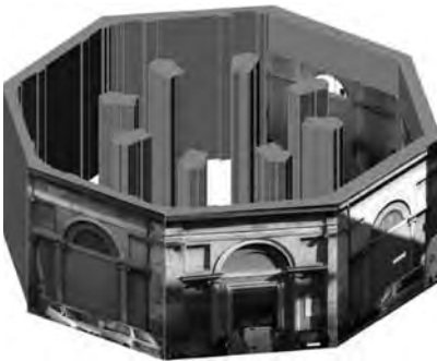
Fig. 3 Laboratory of architectural restoration, a.a. 2006-2007, prof. N. Lombardini From the top: material decay survey; structural decay survey; 3D model and rectified images of the façades. Students: Carolina Lucaccioni, Giorgia Menozzi, Silvia Peragine.
